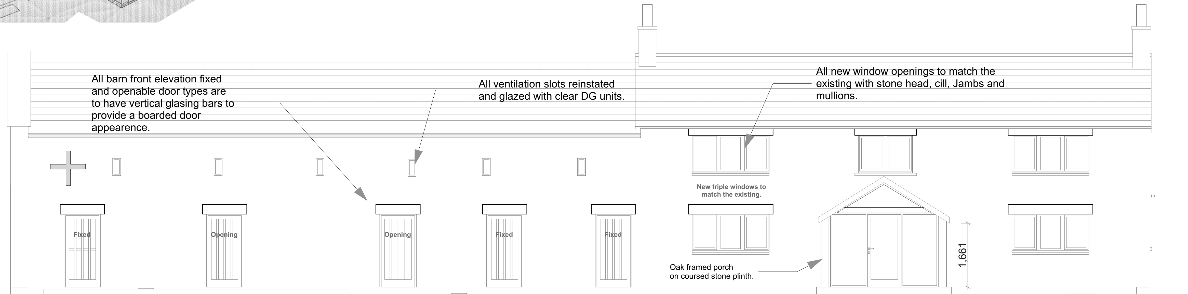
South Elevation 1:50 Elevation
