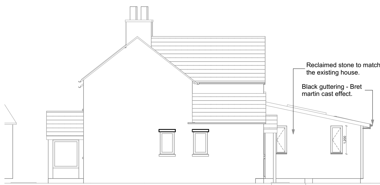
East Elevation 1:100 Elevation
