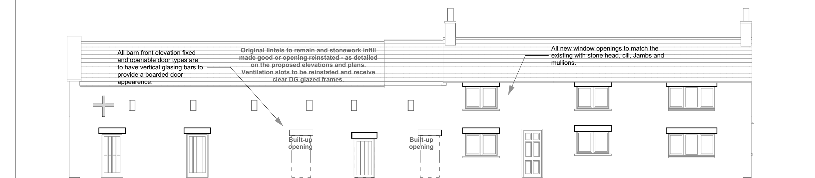
South Elevation Elevation 1:100
